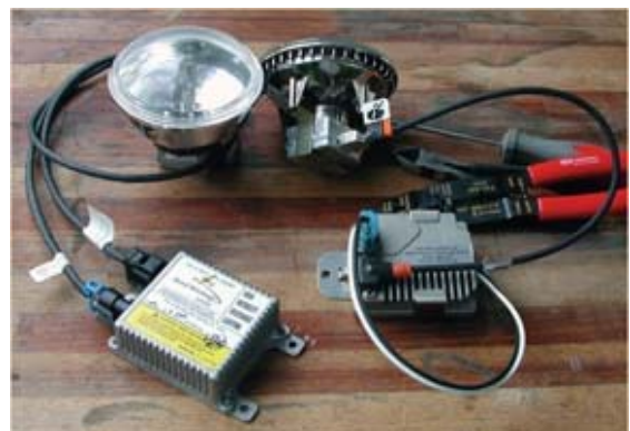
HIDs ready for trials, above. LoPresti Boom Beam, left, is for a Cessna 210. Knots2U system, right, fits a variety of
