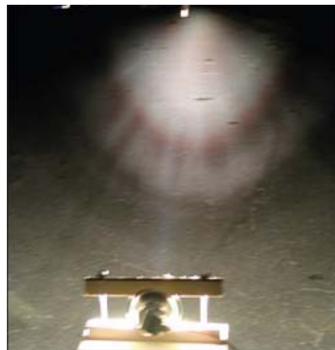
XeVision's 50-watt system, above, was the brightest of any of the HIDs tested.
